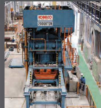
The cutting-edge full automatic 20,000 ton Press machine
